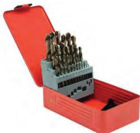
5% cobalt steel 25-piece drill bit set. Ideal for hard to drill metals such as hardened steel, cast iron, titanium and stainless steel as it is more resistant to high temperatures. Contains: 1, 1.5, 2, 2.5, 3, 3.5, 4, 4.5, 5, 5.5, 6, 6.5, 7, 7.5, 8, 8.5, 9, 9.5, 10, 10.5, 11, 11.5, 12, 12.5 & 13 mm.
