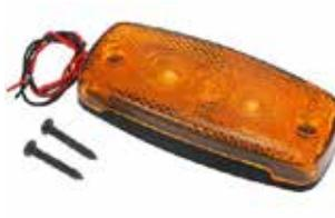
Amber front LED marker lamp/reflector. Length 108mm Width 50mm Depth 20mm. Bolt holes 5mm diameter. Bolt hole centres 83mm.
