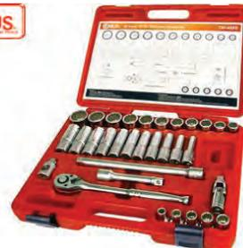
1/2" drive set in a HD plastic case. Including 27 12-point hand and deep hand sockets from sizes 3/8" to 1 1/4" and 3/8" to 7/8" respectively, a two way adapter (3/8" female to 1/2" male), 5" and 10" long extension bars, universal joint and a quick release ratchet.
