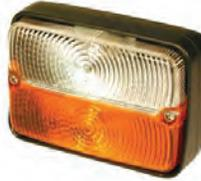
Amber flasher. White side light. Complete with bulbs. Suitable for Massey Ferguson 3000, 3100, and 3600 series & Deutz applications. Replacement bulbs: 1 x VLC0382, 1 x VLC0207. VPM3711 lens.
