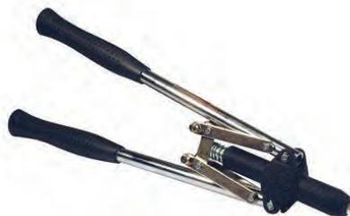
Industrial compound action hand riveter with high leverage long tubular steel handles. Head with nozzles to accept 3.2m 4.0 and 4.8mm aluminium alloy, stainless steel blind rivets.
