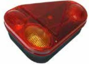
Left hand rear five function lamp. Stop/tail/indicator/fog and reflective triangle. Length 230mm, Width 180mm Depth 60mm. Replacement bulb: VLC0382 x 2 and VLC0380 Replacement lens VLC2305
