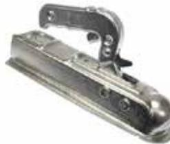
A galvanised 50mm ball coupling for unbraked trailers up to 750 kg. Fits a 50mm square drawbar. M12 diameter bolts to a tensile strength of class 8.8 must be used to connect the coupling head to drawbar. For example VLG1859 M12 x 70mm bolt & VLG4236 M12 Nylon Lock Nut
