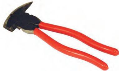
Manufactured from specially selected steel with a smooth ground head. These 10" fencing pliers have a maximum jaw opening of 35mm, these fencing pliers can cut, splice and stretch wire in addition to pulling and driving staples. 240mm long
