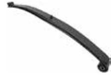
Parabolic road springs. Fitted to some Ifor Williams trailers manufactured after 1994. Length following curve of spring 800mm. Width 50mm. 12mm Diameter hole in metal spring bush.
