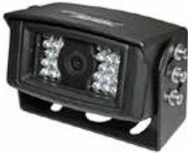
The VLC5067 wired camera is an IP69 rated waterproof colour CCD camera with audio, 110 degrees of viewing angle and 28 infrared illuminators for night vision up to 32 feet (10m). The VLC5067 also has day/night sensors for automatic light adjustment, mirroring capabilities and is built to withstand off-road conditions.
