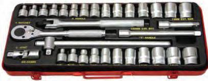
32 piece 3/8" drive metric & AF hand socket set in a HD steel case comes complete with 6mm to 19mm, 21mm and 1/4" to 7/8" sockets, 75mm and 150mm long extension bars, sliding t-handle, universal joint, reversible ratchet handle and a hinge handle.
