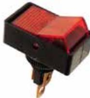
Medium duty (On / Off) red illuminated rocker switch with 3 terminals. 12 Volt, 16 Amp. Fitted with a 12 Volt bulb. Requires a 12mm diameter mounting hole and for use with panels up to 4mm thick.
