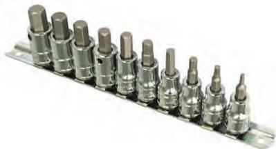
3/8" drive set with a wall mountable steel socket holder, this 10 piece metric hex bit socket set contains sockets 3mm, 4mm, 5mm, 6mm, 7mm, 8mm, 9mm, 10mm, 11mm and 12mm. Made of high speed tool steel.
