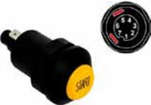
12 / 24 Volt 25 Amp switch with yellow lens and black marking: START. 2 pin connection. Requires 31mm mounting hole and for use with panels up to 5.5mm thick.
