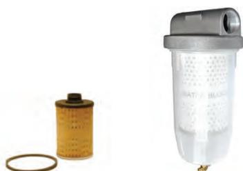
Fuel tank filter unit. For use with petrol, diesel, and other fuels. Removes microscopic contaminants to 10 microns. Heavy duty metal housing with 1" BSP ports. Impact resistant plastic bowl with a working pressure of 150psi/10 Bar and fitted with a drain valve. Replace filter element after 12 months (recommended).
