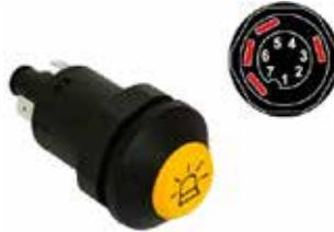
12 Volt 25 Amp illuminated switch with yellow lens and black marking for rotating beacons. Supplied with 12 Volt bulb and has a 4 pin connection. Requires 31mm mounting hole and for use with panels up to 5.5mm thick.
