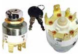
Supplied with 2 keys. Park / Off / On / Ignition. Start circuit 12 Volt 30 Amp, ignition and accessory circuit 12 Volt 10 Amp. Chrome plated. Requires 18.8mm mounting hole and for use with panels up to 8mm thick.
