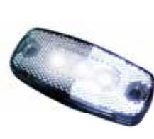
Clear front LED marker lamp/reflector. Length 108mm Width 50mm Depth 20mm. Bolt holes 5mm diameter. Bolt hole centres 83mm.
