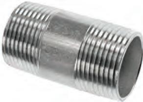
1" BSP male - male fitting, galvanised steel for weather protection suitable for use with VLA3006 and VLA3058 filter assemblies. Use PTFE thread tape for sealing during fitment.
