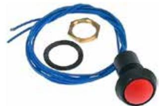
12.5 Volt 125 mA push button switch. Requires 13.2mm mounting hole and for use with panels up to 2.3mm thick. Suitable for use with VFH1009 12.5V, 125 mA push button switch.
