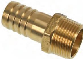
Brass 1" BSP - 1" (25.4mm) hose tail to fit 1" i/d fuel delivery hose. Use PTFE thread tape for sealing during fitment.
