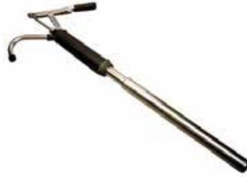
Hand lever operated metal barrel pump. Telescopic suction tube permits operation on barrels from 490mm to 865mm deep. Standard 2in BSP thread. Delivery 260ml per stroke.
