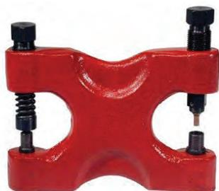
Eze rivet tool assembly for simple and rapid on-site repairs to cutter bars on combine harvesters, mowers and hedge trimmers. Precise rivet expansion is ensured to give durable and permanent knife section replacement.
