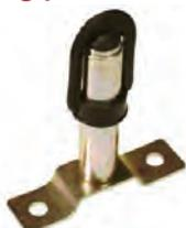
Bolt on mounting pole for rotating beacons. Overall height 110mm, boltholes 10mm, bolt hole centres 85mm.
