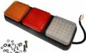
Complete LED modular rear combination lamp with stop/tail, indicator and reverse functions. Rubber base. Varivolt 10-30v. Length 275mm Width 95mm Depth 35mm. Replacement stop/tail module VLC2317. Replacement indicator module VLC2309. Replacement reverse module VLC2318.
