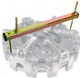
When rebuilding and fitting a dual clutch assembly it is important to ensure that the clutch release levers are correctly set. This bridging tool allows quick and simple height alignment of all levers so preventing premature release bearing or clutch plate failure. For Massey Ferguson.
