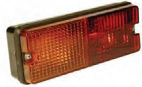
Rear lamp. Amber flasher. Bulbs not supplied. Red side/brake light. Suitable for some Zetor applications. Use 2 x VLC0382 bulbs & VPM3736 lens.
