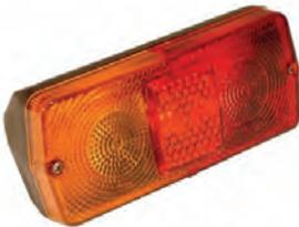
Amber flasher. Red side/brake light. Bulbs not supplied. Suitable for some Massey Ferguson 500 series applications. Use with 1 x VLC0380, 1 x VLC0382 bulbs.
