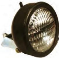
Rubber cased light. Sealed beam. Complete with switch. 12 volt, 35 watt. 130mm dia. Replacement sealed beam unit: VLC2007.
