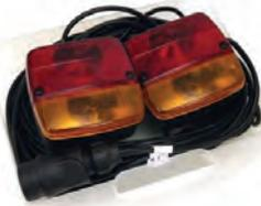
Consists of two 12 Volt magnetic mounting, 4 function rear trailer lights with 4m of cable between them and 12m of cable fitted with a 7 pin plug. This product comes in a useful plastic carry case for easy storage and enhanced point of sale display. Comes complete with 2 x VLC0382, 2 x VLC0380 bulbs. Uses replacement VLC6011 unit & VLC6010 lens.
