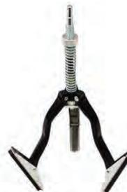
The 3 leg cylinder hone has an adjustable spring tension for positive cutting action which enables smooth honing at all speeds. The spread limiter permits easy insertion into cylinder. 51-177mm (2" - 7").
