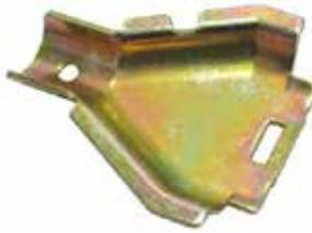
Half shell to support cable entry into brake backplate on Al-ko type back plates. Ifor Williams trailers would be fitted with a 73mm black plastic knock in hub cap.
