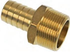
Brass 1 1/4" BSP - 1" (25.4mm) hose tail to fit 1" i/d fuel delivery hose. Use PTFE thread tape for sealing during fitment.
