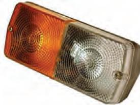
RH side. Bulbs not supplied. Amber flasher. White side light. Wired. Suitable for some Massey Ferguson 200 series applications. Use with 1 x VLC0382, 1 x VLC0207. Uses VPM3672 replacement lens.
