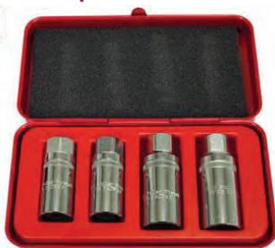
This 1/2" drive AF stud puller set allows you to remove studs without damage to surrounding machinery. The harder you turn, the harder they grip so you can remove even the tightest of studs. Made from chrome vanadium steel and presented in a sturdy metal case. Sizes : 1/4, 5/16, 3/8 and 7/16" (Box : 190x100mm).
