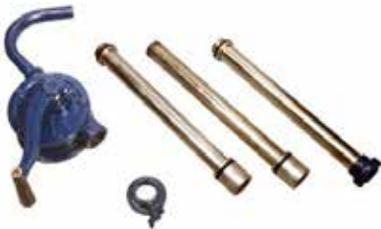
Robust metal construction. Suitable for fuels and light oils. 2" BSP retention adaptor, 980mm steel suction tube and discharge spout. Delivery 410ml per rotation.
