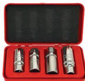
This 1/2" drive metric stud puller set allows you to remove studs without damage to surrounding machinery. The harder you turn, the harder they grip so you can remove even the tightest of studs. Made from chrome vanadium steel and presented in a sturdy metal case. Sizes : 6, 8, 10 and 12mm (Box : 190x100mm).
