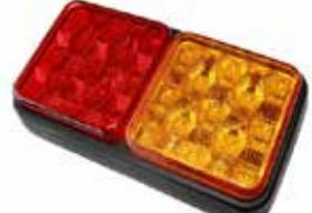
LED modular 3 function (stop/tail & indicator) rear combination lamp. Rubber base. Varivolt. Length 174mm Width 94mm Depth 32mm. Replacement modules are VLC2317 stop/tail and VLC2309 indicator
