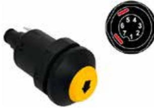
12 / 24 Volt 25 Amp switch with yellow lens and black marking: Lift / lower. 2 pin connection. Requires 31mm mounting hole and for use with panels up to 5.5mm thick.
