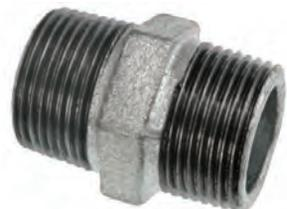
1" BSP male - male fitting, galvanised steel for weather protection. Use PTFE thread tape for sealing during fitment.
