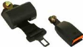
Emergency locking retractor (ELR) 2 points, fully retractable. Dual sensitive (webbing and retractor acceleration). Webbing capacity of ELR is 1000mm
