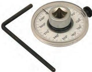
Designed for use on engines when an additional angular rotation movement is specified after torque loading is achieved can be used with any 1/2" drive wrench.
