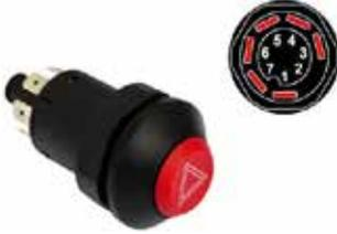
12 Volt 25 Amp illuminated switch with Red lens and white marking: Hazard. Supplied with 12 Volt bulb and has a 6 pin connection. Requires 31mm mounting hole and for use with panels up to 5.5mm thick.
