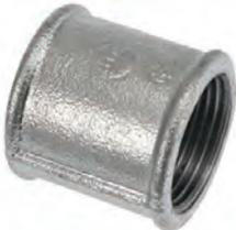
1" BSP female socket, galvanised steel for weather protection. Use PTFE thread tape for sealing during fitment.
