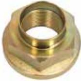
Stake nut with flange that can also be used as replacement to stake nut and washer. Requires 45mm socket or spanner. Overall outside diameter 58mm. Overall thickness 30mm. Commonly found on Ifor Williams trailers manufactured after 1994. It is recommended to replace stake nuts after each removal. Ifor Williams trailers using stake nuts would have 75mm black or 76mm grey plastic knock in hub caps.
