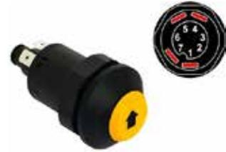
12 / 24 Volt 25 Amp switch with yellow lens and black marking: Lift / lower. 4 pin connection. Requires 31mm mounting hole and for use with panels up to 5.5mm thick.
