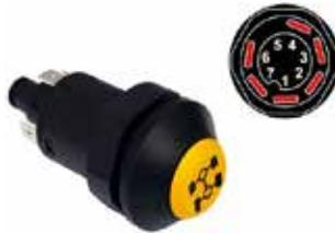
12 Volt 25 Amp illuminated switch with yellow lens and black marking: 4WD. Supplied with 12 Volt bulb and has a 6 pin connection. Requires 31mm mounting hole and for use with panels up to 5.5mm thick.
