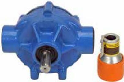
High volume PTO roller-vane pump c/w 1 3/8in 6 spline quick release coupling. Output 147.3l/min at 0 PSI to 93.5l/min at 150 PSI. As used and supplied in VTB1250.
