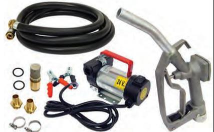
A self-priming pump with built in by-pass for diesel and light oil transfer. 40 litres per minute capacity. Supplied with on/off switch, carrying handle, 2m battery cable with clips, 4m hose, metal nozzle and filter. Requires 12 or 24 volt DC supply.
