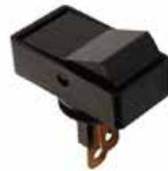
Medium duty (On / Off) rocker switch with 2 terminals. 12 Volt, 16 Amp. Requires a 12mm diameter mounting hole and for use with panels up to 4mm thick.
