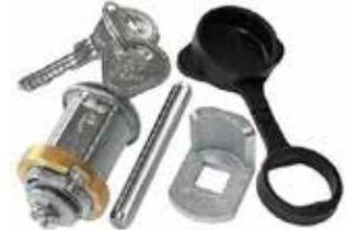
Lock insert for Knott Avonride coupling units. Supplied with two keys. Suitable for KF13 & KF13E, KFG27, KFG35, KF20, KFG20 and KRV20 couplings. Replacement for standard fitment hitch lock. Overall length 57mm Thread diameter 18mm
