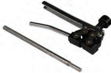
A simple and effective means of breaking roller chain. Simply place the chain into the device and tighten until the pin is removed. Large chain breaker - for chain pitch in range from 1" to 1 1/2".
