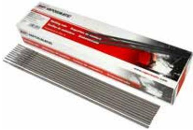
2.5mm diameter. A medium, heavy coated, all position electrode for all major structural works. Produces a smooth, clean deposit with spatter loss and easy slag removal. Suitable for radiographic works. Min 260 rods per pack.
