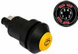
12 Volt 25 Amp illuminated switch with yellow lens and black marking: Windscreen washer. Supplied with 12 Volt bulb and has a 4 pin connection. Requires 31mm mounting hole and for use with panels up to 5.5mm thick.
