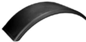
Flexible rubber mudwing suitable for 4wd axles. Width 400mm, Length 1315mm, Radius 720mm, Depth 40mm, Weight 2.7kg.
