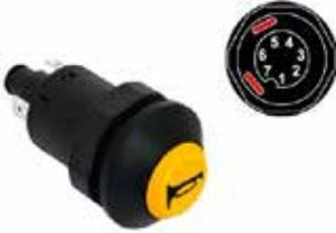
12 / 24 Volt 25 Amp switch with yellow lens and black marking: Horn. 2 pin connection. Requires 31mm mounting hole and for use with panels up to 5.5mm thick.
