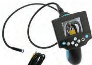
Diagnose faults and problems in seconds with VLA1398 Inspection tool for engine, gearbox, wiring & pipework. Digital photo & video storage enables fault capturing review and reporting. Fixed 9.8mm camera with integral LED illumination & clip-on-tools. Image download via USB port. Video output for connection to TV. Waterproof probe. 512MB memory card included.
