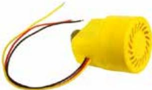
12 - 24 Volt. Includes night time silent reverse. Fully sealed and waterproof. Over voltage and reverse polarity protection. 3 wire connection. Sound level @ 1m = 96db. CE and 'e' marked.
