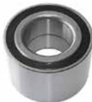
One piece double row bearing rubber sealed both sides. Bearing is equal to reference 1001 IB3464RRS-2 T45887.10. Outer diameter = 64mm Internal Diameter = 34mm Width = 37mm Can be found on Ifor Williams P5, P6e, P7e and BV648 trailer with suspension axles. Trailers will be fitted with either 52mm or 64mm metal knock in hub cap
