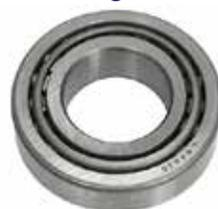
Taper roller bearing L44610 marked on cup. L44643 marked on cone. Commonly used on trailers up to 750 kg including Ifor Williams P6e. Outside Diameter 50mm Inside Diameter 25mm Overall width 15mm
