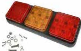
Complete LED modular rear combination lamp with stop/tail, indicator and fog functions. Rubber base. Varivolt 10-30v. Length 275mm Width 95mm Depth 35mm. Replacement stop/tail module VLC2317. Replacement indicator module VLC2309. Replacement fog module VLC2308.
