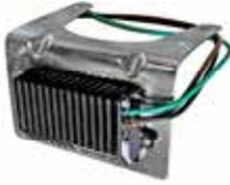
Two required per trailer when fitting LED lamps that provide an indicator function. Suitable for 12 volt circuit only. When trailer LED indicators are working correctly, this relay switches to operate the towing vehicle's audible sensor or dashboard light. Without smart load devices these may not operate due to the negligible load of LED lights.
