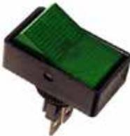
Medium duty (On / Off) green illuminated rocker switch with 3 terminals. 12 Volt, 16 Amp. Fitted with a 12 Volt bulb. Requires a 12mm diameter mounting hole and for use with panels up to 4mm thick.
