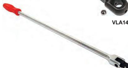
1/2" drive hinge handle. Length of 620mm gives good reach and leverage. An ergonomic, sturdy plastic handle provides ample grip. Made of high quality chrome vanadium steel for strength and long life operation.
