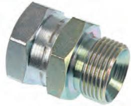
1" BSP male /female swivel type fitting to enable correct positioning of filter assemblies. Use PTFE thread tape for sealing during fitment.
