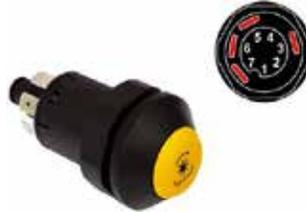
12 Volt 25 Amp illuminated switch with yellow lens and black marking: PTO engagement. Supplied with 12 Volt bulb and has a 4 pin connection. Requires 31mm mounting hole and for use with panels up to 5.5mm thick.
