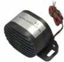
Carefully optimised frequency/loudness characteristics make these units clearly audible under typical working conditions without being a nuisance in the urban/highway environment. Sound Level dB(A) @1m :90°. Conform to SAE J994. CE and 'e' marked.
