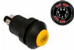
12 Volt 25 Amp illuminated switch with yellow lens and black marking: Start. Supplied with 12 Volt bulb and has a 4 pin connection. Requires 31mm mounting hole and for use with panels up to 5.5mm thick.
