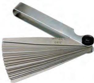
20 piece feeler gauge set. Hardened, tempered and polished steel blades. Folds into a steel case for added protection. Locking screw allows blades to be held in position. Size etched on to all blades. Size 1.00mm – 0.05mm.
