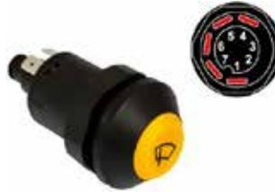
12 Volt 25 Amp illuminated switch with yellow lens and black marking: Windscreen wiper. Supplied with 12 Volt bulb and has a 5 pin connection. Requires 31mm mounting hole and for use with panels up to 5.5mm thick.
