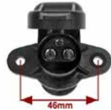
3 pin power socket with a two hole mounting flange (46mm centres). Requires 26mm mounting hole for body.
