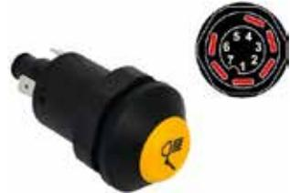
12 Volt 25 Amp illuminated switch with yellow lens and black marking: Work light. Supplied with 12 Volt bulb and has a 4 pin connection. Requires 31mm mounting hole and for use with panels up to 5.5mm thick.
