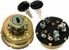
Starter switch. Fiat type. Requires 21.8mm mounting hole and for use with panels up to 10.5mm thick.
