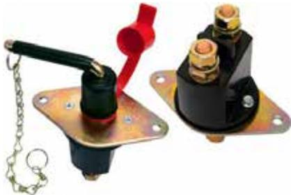
Heavy duty 12 / 24 Volt, 250 Amp, TIR specification switch with removable key. Maximum Current: 2500 Amp for 5 sec.
