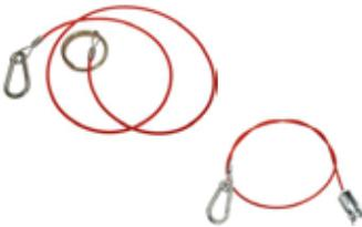
Breakaway cable with spring ring attachment. It is a requirement that braked trailers are fitted with a breakaway cable. This cable will apply the hand brake if for any reason the trailer becomes detached during towing. This cable should be regularly inspected and replaced if any defects are visible.
