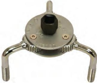
This clever little oil filter wrench attaches to a 3/8" drive ratchet handle and the design allows for broad range and tremendous gripping power. Fits easily into tight spots and features heavy duty grooved legs for a more positive grip. Fully adjustable from 65-110mm (2 1/2" - 4 5/16").
