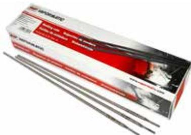
4mm diameter. A medium, heavy coated, all position electrode for all major structural works. Produces a smooth, clean deposit with spatter loss and easy slag removal. Suitable for radiographic works. Min 85 rods per pack.
