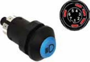
12V, 25 Amp illuminated switch with blue lens and black marking: Full Beam. Supplied with 12V bulb and has a 5 pin connection. Requires 31mm mounting hole and for use with panels up to 5.5mm thick.
