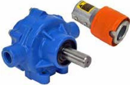
PTO roller-vane pump c/w 1 3/8in 6 spline quick release coupling. Output 53.4l/min at 0 PSI to 31.6l/min at 300 PSI. As used and supplied in VTB1050.
