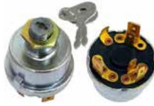
Starter switch. Case - International / David Brown / Leyland Marshall type. Requires 15.4mm mounting hole and for use with panels up to 3.7mm thick.
