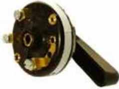
Lever operated (On / Off / On) rotary switch with screw terminals. 12 Volt, 8 Amp. Suitable for indicator applications. Requires a 26.5mm mounting hole and for use with panels up to 4mm thick.
