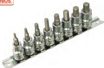
1/2" drive set with a mountable steel socket holder, this 8 piece metric hex bit socket set contains sockets 4mm,5mm,6mm,7mm,8mm,9mm,10mm,12mm. Made of high speed tool steel.
