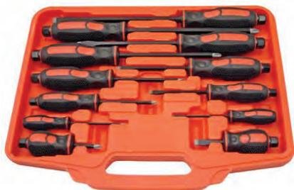
Satin black, chrome vanadium steel blades. Hardened and tempered tips. Polypropylene handles for exceptional grip. Slot size: 9.5x200mm, 8x100mm, 6x100mm, 5x75mm, 3.2x75mm, 6x38mm. Phillips size: 4x200mm, 3x150mm, 2x100mm, 1x75mm, 0x75mm, 2x38mm.
