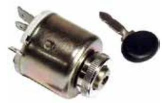
Starter switch. Fiat type. Requires 21.5mm mounting hole and for use with panels up to 4.2mm thick.
