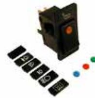
Heavy duty (On / Off) illuminated rocker switch with 4 terminals - for use with relay. 12 Volt, 20 Amp. Fitted with 12 Volt bulb. Supplied with 4 colour discs and various symbols for universal applications. Requires 38.7x18.5mm mounting hole and for use with panels up to 3.8mm thick.
