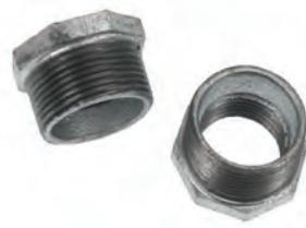
11/4" BSP male - 1" BSP female reducer for use with VLA3061 and VLA3062. Galvanised steel for weather protection. Use PTFE thread tape for sealing during fitment.
