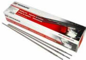
3.15mm diameter. A medium, heavy coated, all position electrode for all major structural works. Produces a smooth, clean deposit with spatter loss and easy slag removal. Suitable for radiographic works. Min 170 rods per pack.
