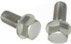
M14 x 1.5mm pitch. 19mm head diameter. Thread length 27mm, Overall length 45mm. Fitted to trailers with Knott 250mm x 40mm type brakes. Wheel bolts should be torqued to 110Nm.
