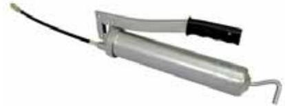
A Metric Load-a-matic grease gun. Can be bulk loaded or used with 400g cartridges. Complete with 30cm flexible extension pipe and 4 jaw M10 coupler. Operating pressure 705 bar. Use VLB1027 couplers and VLB1029/VLB1041 flexi pipes as suitable replacements.
