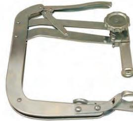
For the rapid and safe removal of valve springs and collets from petrol and diesel engines with deep seated valves. Size 255mm with an adjustable jaw capacity ranging from: 66 - 194mm. Throat depth 242mm.
