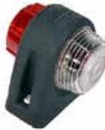
Britax rubber body front and rear marker lamp. 12volt. Red and clear lenses. 70mm hole centres. Replacement bulb: VLC0207. Replacement lenses- Red = VLC2275 Clear = VLC2332
