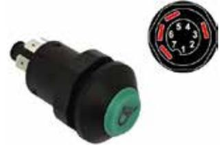
12 Volt 25 Amp illuminated switch with green lens and black marking: Side lights. Supplied with 12 Volt bulb and has a 4 pin connection. Requires 31mm mounting hole and for use with panels up to 5.5mm thick.
