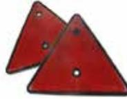
Reflective triangle less white surround. Dimensions Height 140mm Width 160mm Hole Centres 70mm Hole diameters 5mm
