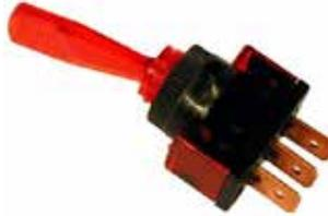
2 position (On / Off) illuminated toggle switch suitable for 12 Volt applications up to 20 Amps. Requires 11.5mm mounting hole and for use with panels up to 3.3mm thick.
