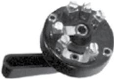
Lever operated 4 position (0, 1, 1+2, 1+3) rotary switch with screw terminals. 12 Volt, 8 Amp. Suitable for vehical lighting applications. Requires a 26.5mm mounting hole and for use with panels up to 4mm thick.
