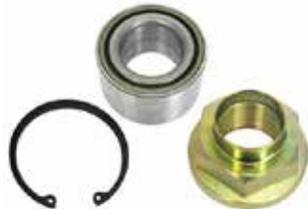
Wheel bearing kit. Fits Ifor Williams trailers manufactured after January 1994. Trailers would be fitted with either 75mm black plastic or 76mm grey plastic knock in hub cap. Kit includes wheel bearing, bearing retaining circlip and stake nut. Stake nut should be tightened to 350Nm.
