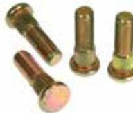
3/8" UNF thread. 22mm thread length, 10.4mm diameter over splines. Commonly used on trailers up to 750kg including Ifor Williams P6e. To be used with VPN4012 wheel nut.
