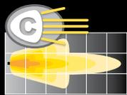
Combo lighting provides 'versatility' by combining both spot beam with flood beam patterns, all within the same light. Combo lighting provides simultaneous long distance terrain lighting together with closer field illumination. However, without separate beams neither the flood or spot light patterns are as bright as a dedicated spot or flood beam light.
