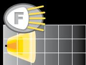
Flood lighting generally has a short but wider 60-90 degree beam pattern for more even light dispersal over a greater area. Flood illumination is ideal when you need to light up a given work area and helps provide excellent close working-quarter illumination.
