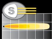
A spot light beam has a narrow illumination spread of typically 8 degrees. By focusing the light beam in a narrow area makes this type of longer distance lighting ideal for specific tasks, sprayer boom applications or highlighting the forward driving path.
